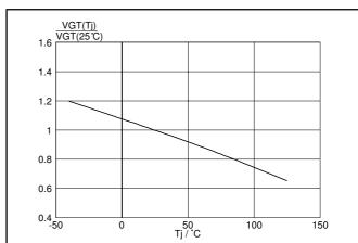
Fig.6. Normalised gate trigger voltage  $V_{GT}(T_i)/V_{GT}(25^{\circ}C)$ , versus junction temperature  $T_i$ .
