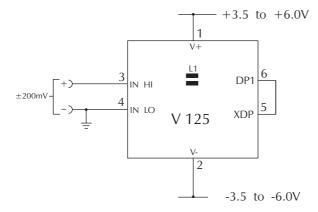
Measuring a single ended input referenced to supply, i.e. the input voltage and the meter's power supply share the same 0V rail. Check Link L1 is open.
