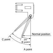
Output voltage between A point and C point shall be from low level to high level when the actuator level rotated  $(37^{\circ} \pm 5^{\circ})$  from normal condition B point to C point in Fig.1. Normal condition B point shall be opaque condition.
