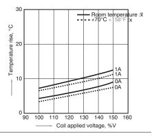
5-(2). Coil temperature rise Tested sample: TXS2-24V, 6 pcs. Point measured: Inside the coil
