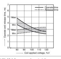
6-(2). Operate and release time (without diode) Tested sample: TXS2-4.5V, 10 pcs.
