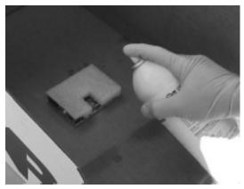
Figure 5. Applying Coating to Masked Board
