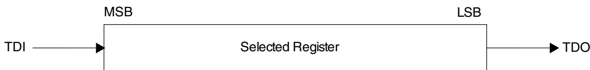
Figure 56-3. Shifting data through a register
