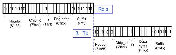
Figure 6: Master's Read Packet Structure
