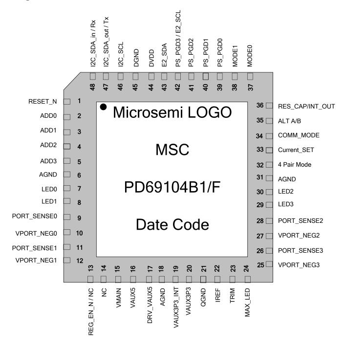
PD69104B1 for -10° to +85°C Operating Ambient Temperature Range PD69104B1F for -40° to +85°C Operating Ambient Temperature Range
