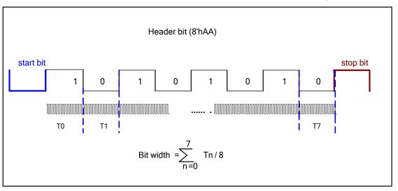
Figure 8: Header Bit Width
