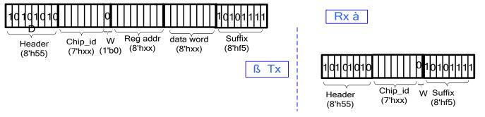
Figure 7: Master's Write Packet Structure
