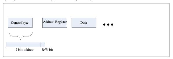
Figure 3: High Level Packet Structure
