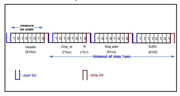
**Figure 9: Timeout Mechanism**
