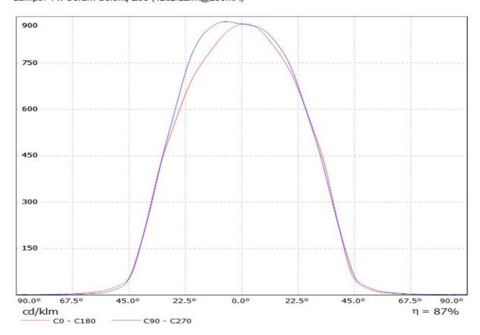
Luminaire: LEDiL Oy CN13112\_LENINA-W\_(SoleriqE30) Eff.86.8% Lamps: 1 x Osram Soleriq E30 (1262.22lm@250mA)
