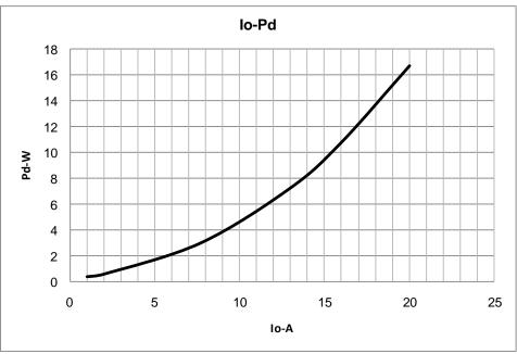
Thermal resistance calculation formula for Heat sink is as follows: Rth = (Tc-Ta)/Pd
