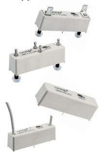
Recently approved by UL, very high isolation voltages (up to 10kV) are achieved through the use of high vacuum reed switches with Tungsten contacts and make these relays suitable for high reliability applications, such as cardiac defibrillators, test equipment and high voltage power supplies.
