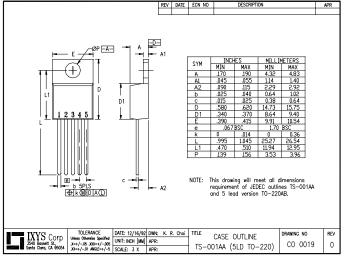
NOTE: Mounting or solder tabs on all packages are connected to ground
