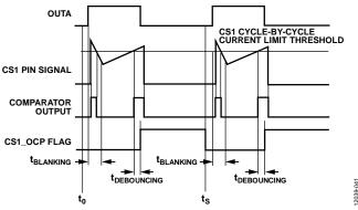
Figure 35. CS1 Cycle-by-Cycle Current-Limit Timing
