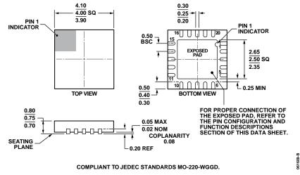
Figure 59. 20-Lead Lead Frame Chip Scale Package [LFCSP\_WQ] 4 mm × 4 mm Body, Very Very Thin Quad (CP-20-10) Dimensions shown in millimeters
