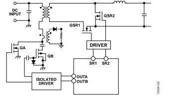
Figure 11. PWM Assignment for Active Clamp Forward Topology with Synchronous Rectification
