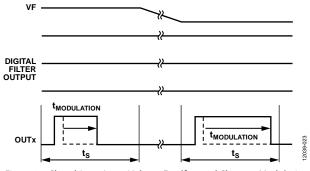
Figure 21. Closed-Loop Input Voltage Feedforward Changes Modulation Values
