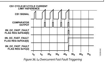
For the single-ended topologies, such as forward converter and buck converter, a switching cycle consists of one cycle. For the double-ended topologies, such as full bridge converter, half bridge converter, and push pull converter, there are two cycles in a switching cycle. The IIN\_OC\_FAST\_FAULT\_LIMIT bits are in Register 0xFE1A[6:4]. In Figure 36, the IIN\_OC\_FAST\_ FAULT\_LIMIT value is set to 8.
