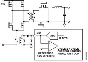
Figure 23. Current Sense 1 (CS1) Operation
