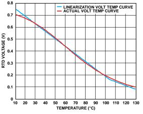
Figure 32. Temperature Linearization Scheme Curves
