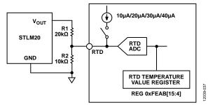
Figure 30. Temperature Sensing by an Analog Temperature Sensor
