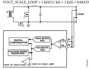
Figure 18. Voltage Sense Configuration
