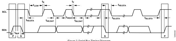
Figure 2. Serial Bus Timing Diagram
