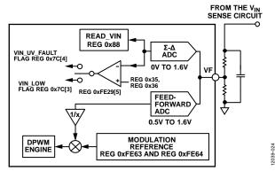
Figure 22. Open-Loop Feedforward Operation
