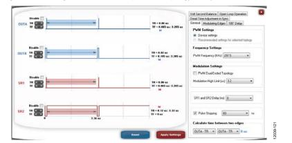
Figure 12. PWM Settings for Active Clamp Forward Topology with Synchronous Rectification Using the ADP1050 GUI
