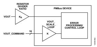
Figure 54. Conceptual View of the VOUT\_SCALE\_LOOP Command
