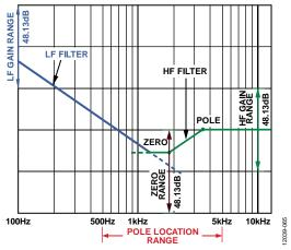
Figure 56. Digital Compensator Programmability
