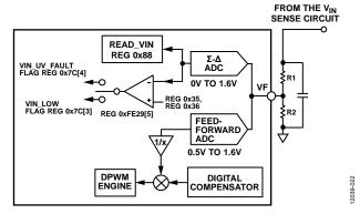
Figure 20. Closed-Loop Input Voltage Feedforward Configuration
