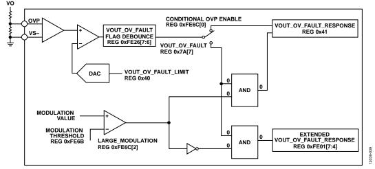
Figure 33. VOUT Overvoltage Protection Circuit Implementation
