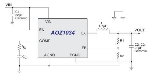
Figure 1. 3.3V 4A Synchronous Buck Regulator
