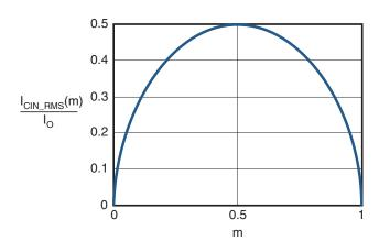
Figure 2. I<sub>CIN</sub> vs. Voltage Conversion Ratio
