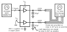
FIGURE 2. Simultaneous Switching Test Circuit
