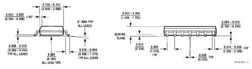
14-Lead Small Outline Integrated Circuit (SOIC), JEDEC MS-120, 0.150" Narrow Body Package Number M14A
