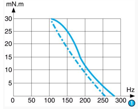
Max. stopping-starting and operating curves at I constant (PBL 3717) for 2 (motor) phases 10.7 ohms. Holding torque 70 mN.m Current per phase 0.59 A
