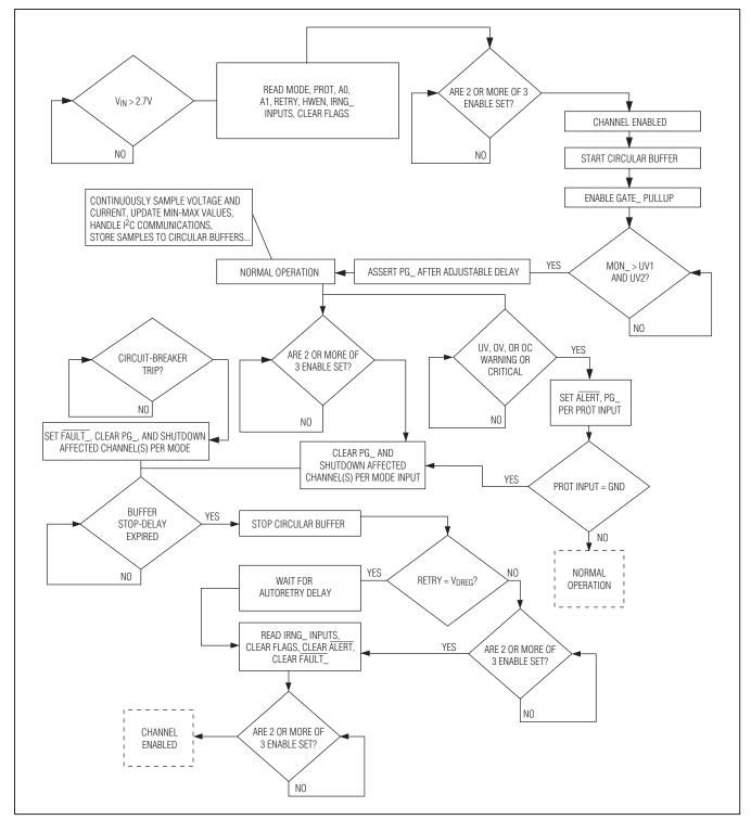
Figure 2. Operation and Fault-Management Flowchart for One Channel
