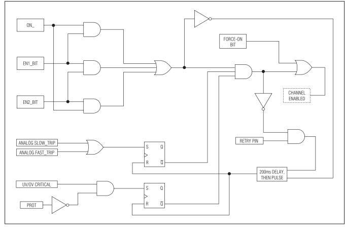
Figure 1. Channel On-Off Control Logic Functional Schematic
