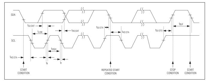
Figure 4. Serial-Interface Timing Details
