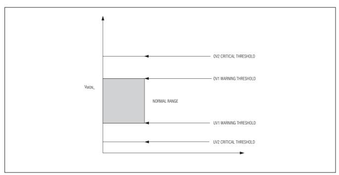
Figure 3. Graphical Representation of Typical UV and OV Thresholds Configuration
