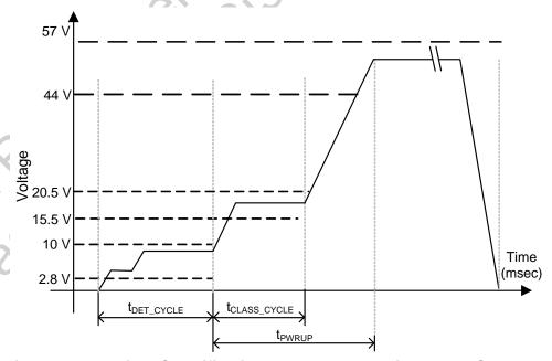
Figure 2. Detection, Classification, Powerup, and Disconnect Sequence
