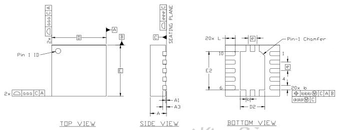
Figure 4. QFN-11 Package Drawing
