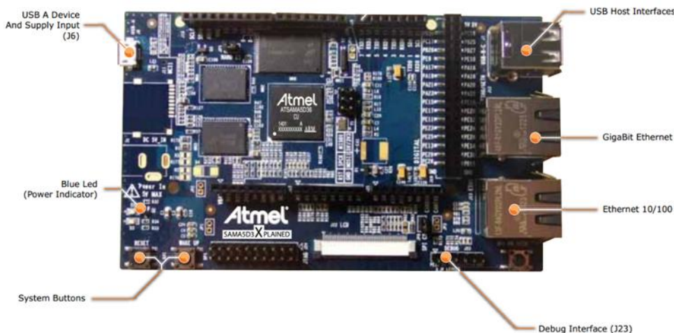
Figure 2-2. SAMA5D3 Xplained Board Overview
