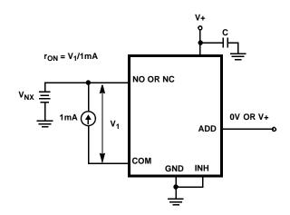
FIGURE 5. ron TEST CIRCUIT
