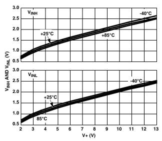
FIGURE 11. DIGITAL SWITCHING POINT vs SUPPLY VOLTAGE
