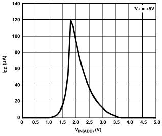
FIGURE 12. SUPPLY CURRENT vs DIGITAL ADDRESS INPUT VOLTAGE
