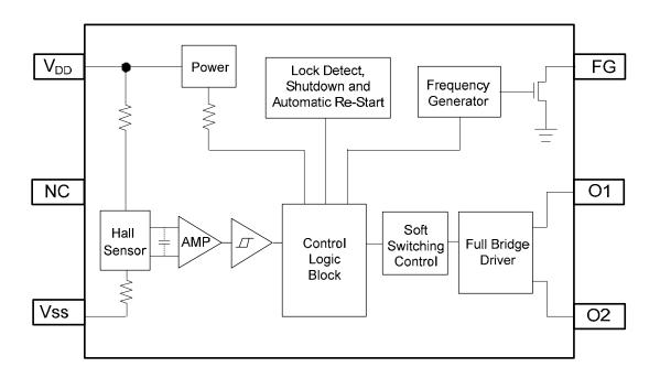
Notes: 2.The AH5794 has an open-drain tachometer FG output that follows the magnetic change frequency. Typically a pull-up resistor of 10kΩ is recommended from FG pin to the supply voltage.
