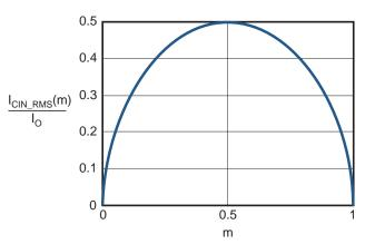
Figure 2. I<sub>CIN</sub> vs. Voltage Conversion Ratio
