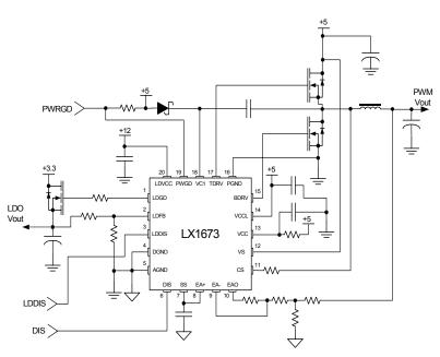
Figure 3 – Schematic with Bootstrap Supply for PWM High Side Drive
