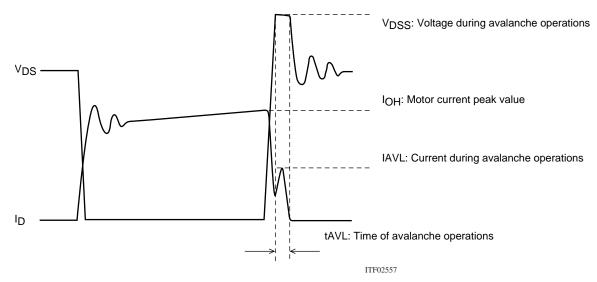
Figure 1 Output Current, I<sub>D</sub>, and Voltage, V<sub>DS</sub>, Waveforms 1 of the STK672-7\*\* Series when Driving a 2-Phase Stepping Motor with Constant Current Chopping
