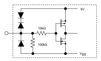
The input pins of this driver all use Schmitt input. Typical specifications at  $Tc=25^{\circ}C$  are given below. Hysteresis voltage is 0.3V (VIHa-VILa).
