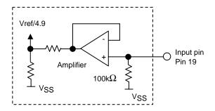
The internal impedance,  $100k\Omega$ , is designed so that the increase in current is prevented while Pin 19 is open. The recommended Vref voltage is 0.14V or higher because the output offset voltage of Vref/4.9 amplifier cannot be controlled down to 0V
