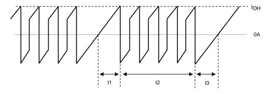
Motor COM Current Waveform Model
