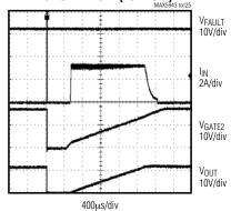
$\begin{array}{l} C_{LOAD}=220\mu\text{F}\\ \text{TIM}=\text{IN} \end{array}$
