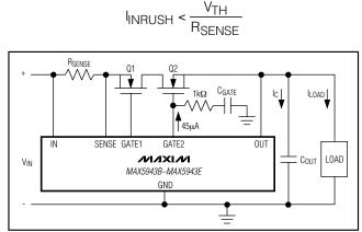
Figure 10. Controlling the MAX5943B-MAX5943E Inrush Current
