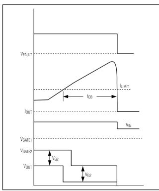
Figure 3. MAX5943B-MAX5943E Circuit-Breaker Timing Diagram
