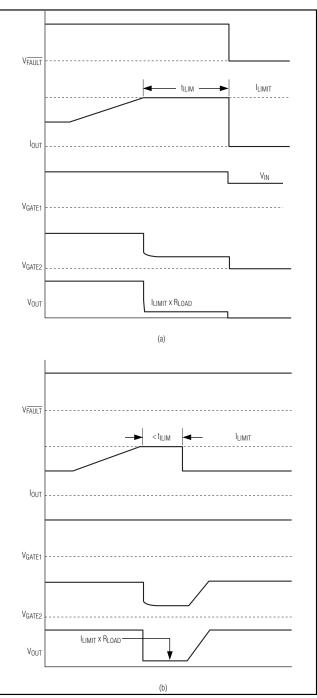
Figure 2. MAX5943A Current-Limit Timing Diagram
