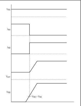
Figure 6. MAX5943 Power Switch Over ORing Timing Diagram
