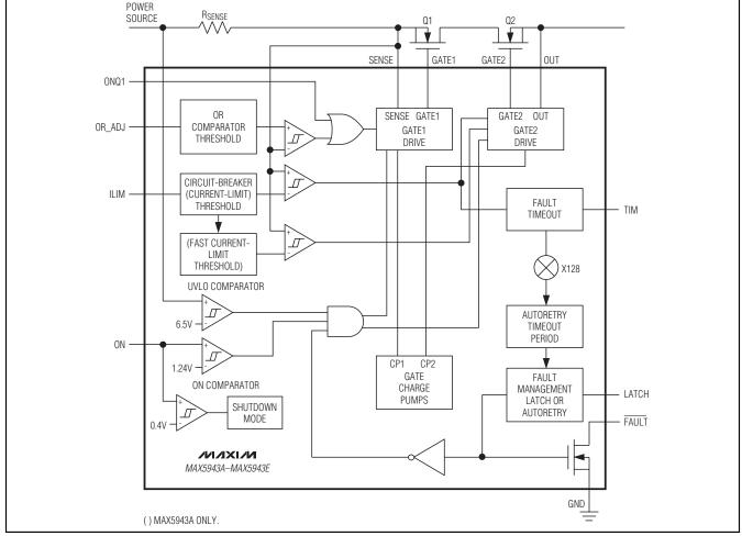
Figure 1. MAX5943 Functional Diagram
