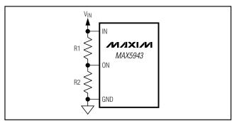
Figure 8. Setting the MAX5943 Turn-On Voltage
