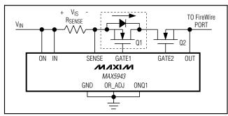
Figure 4. Q1 Current Path During Inital Startup
