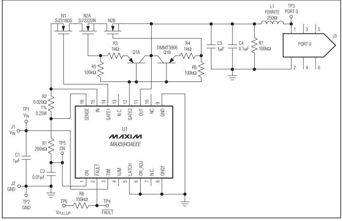
Figure 12. UL-Recognized Single-Port FireWire Protective Circuit
