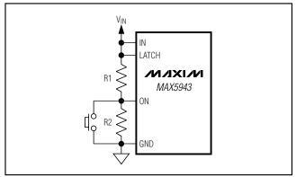
Figure 9. Resetting MAX5943 After a Latched Fault Condition
