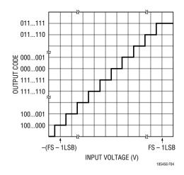
Figure 4. Bipolar Transfer Characteristics
