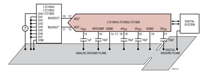
Figure 13. Power Supply Grounding Practice
