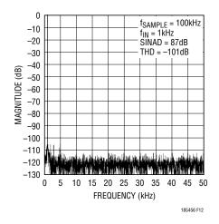
Figure 12. LTC1856 Nonaveraged 4096 Point FFT Plot
