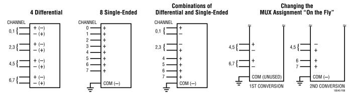
Figure 8. Examples of Multiplexer Options on the LTC1854/LTC1855/LTC1856
