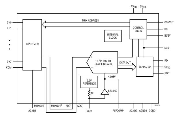
Figure 1. LTC1854/LTC1855/LTC1856 Simplified Equivalent Circuit
