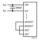
Figure 2. Analog Input Filtering
