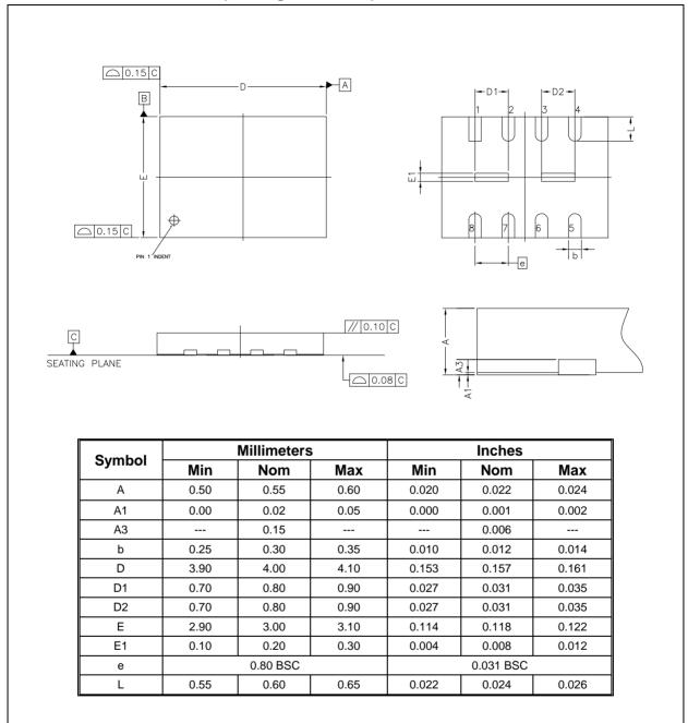
Note:The metal pad area on the bottom center of the package is not connected to any internal electrical signals. It can be left floating or connected to the device ground (GND pin). Avoid placement of exposed PCB vias under the pad.
