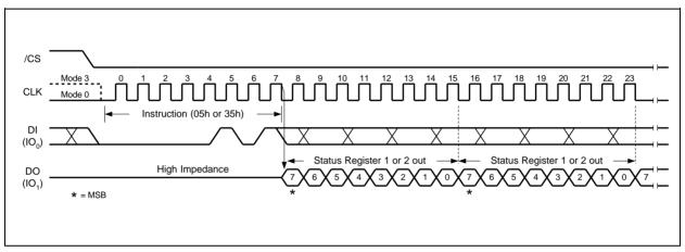
Figure 7. Read Status Register Instruction Sequence Diagram
