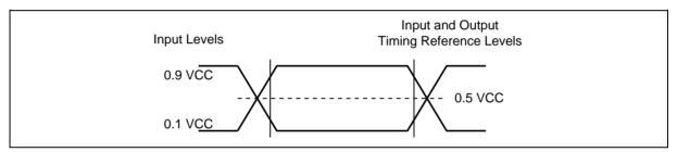
Figure 40. AC Measurement I/O Waveform
