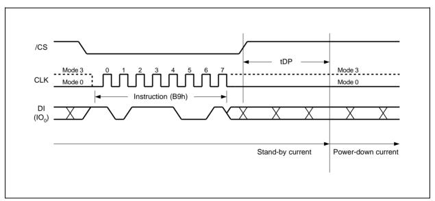
Figure 27. Deep Power-down Instruction Sequence Diagram
