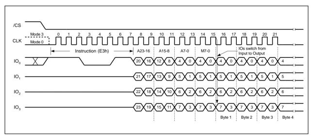
Figure 16a. Octal Word Read Quad I/O Instruction Sequence (Initial instruction or previous M5-4  $\pm$  10)
