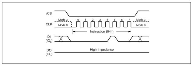
Figure 6. Write Disable Instruction Sequence Diagram
