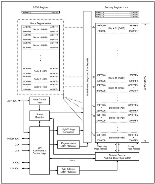
Figure 2. W25Q16DV Serial Flash Memory Block Diagram
