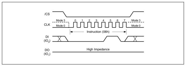
Figure 4. Write Enable Instruction Sequence Diagram
