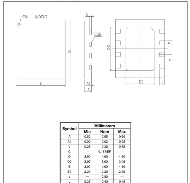
Note:The metal pad area on the bottom center of the package is not connected to any internal electrical signals. It can be left floating or connected to the device ground (GND pin). Avoid placement of exposed PCB vias under the pad.
