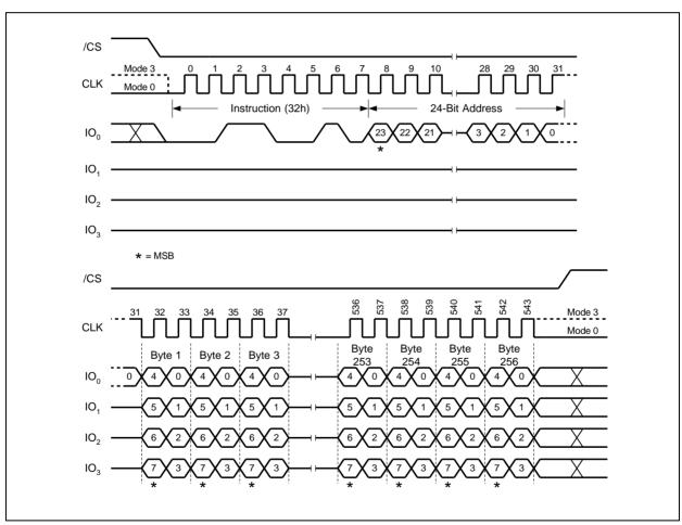
Figure 20. Quad Input Page Program Instruction Sequence Diagram
