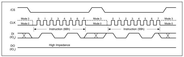
Figure 38. Enable Reset and Reset Instruction Sequence
