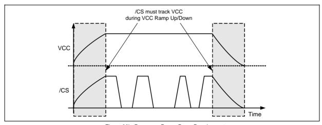
Figure 39b. Power-up, Power-Down Requirement
