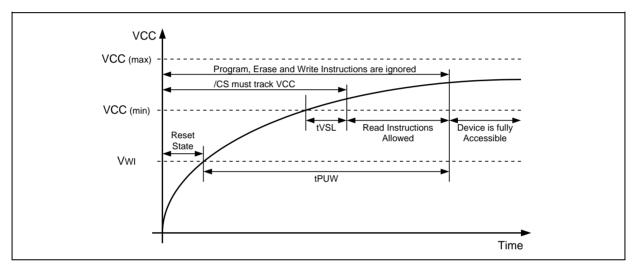
Figure 39a. Power-up Timing and Voltage Levels
