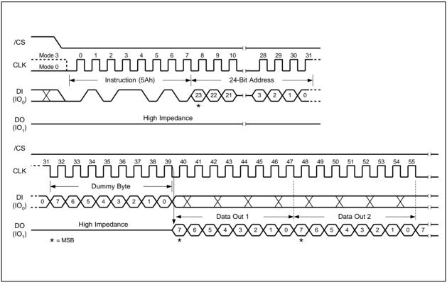
Figure 34. Read SFDP Register Instruction Sequence Diagram
