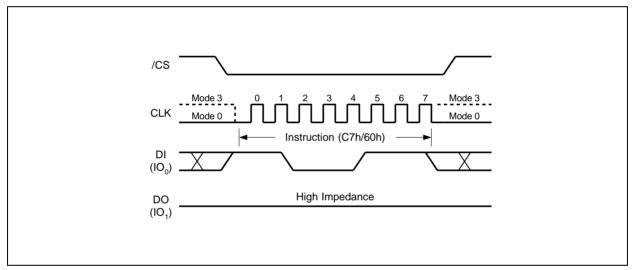
Figure 24. Chip Erase Instruction Sequence Diagram
