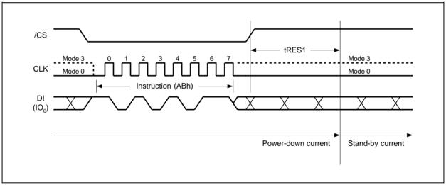
Figure 28a. Release Power-down Instruction Sequence
