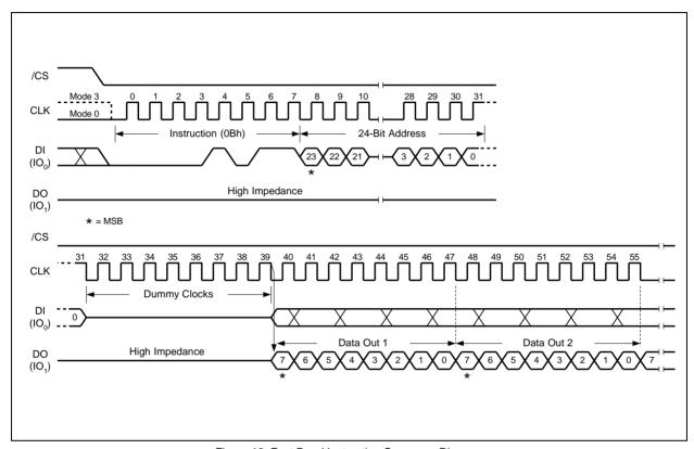
Figure 10. Fast Read Instruction Sequence Diagram
