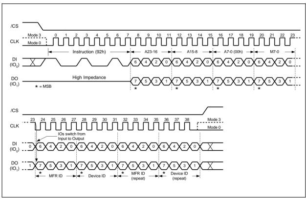
Figure 30. Read Manufacturer / Device ID Dual I/O Diagram
