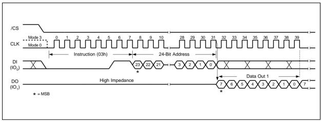
Figure 9. Read Data Instruction Sequence Diagram
