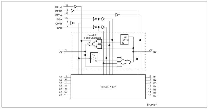
The following examples demonstrate the four fundamental bus-management functions that can be performed with the 74LVT652.
