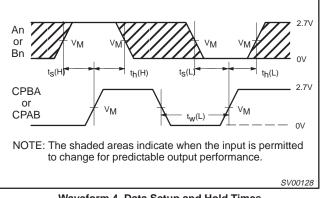
Waveform 4. Data Setup and Hold Times
