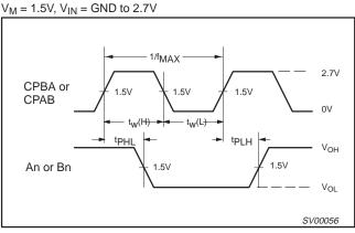
Waveform 1. Propagation Delay, Clock Input to Output, Clock Pulse Width, and Maximum Clock Frequency
