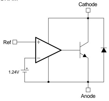
Figure 2 - Simplified block diagram of the IRU431L.
