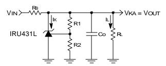
Figure 3 - Typical application of the IRU431L for programming the output voltage.
