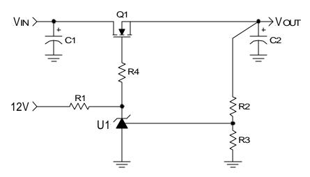
Figure 4 - Low cost 3.3V to 2.7V output.
