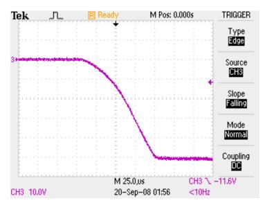
Figure 5. Turn-On Waveform—Vport Relative to GND
