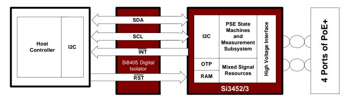
Figure 2. 4-Port System with Direct Host Connection
