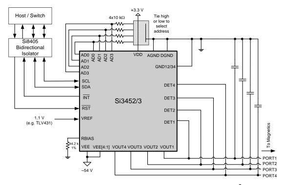
Figure 3. 4-Port Application Diagram Using DC- or dV/dt Disconnect and I<sup>2</sup>C Host Interface
