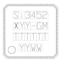
Figure 9. Device Marking Diagram
