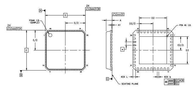
Figure 7. 40-Pin QFN Mechanical Diagram
