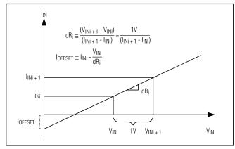
Figure 1. Effective Differential Input Resistance/Offset Current
