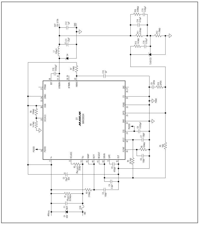
Figure 7. PD with Nonisolated Step-Down (Buck) Converter
