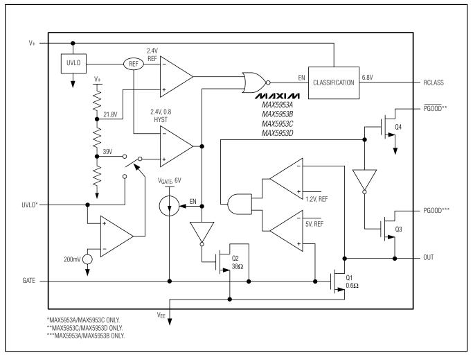
Figure 8. Powered Device Interface Block Diagram
