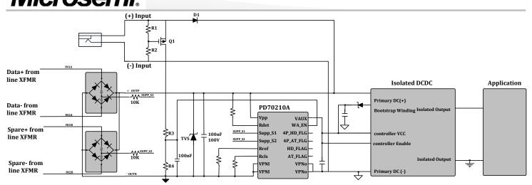
Figure 5: External Power Input connected to PD70210A Output
