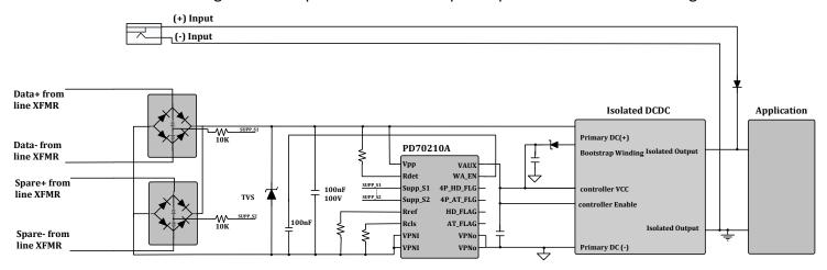
Figure 4: External Power Input connected to Application supply Rails
