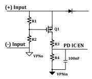
Figure 6: External Power Input resistors dividers
