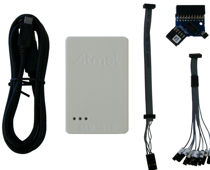
Figure 2-1. Atmel-ICE Full Kit Contents
