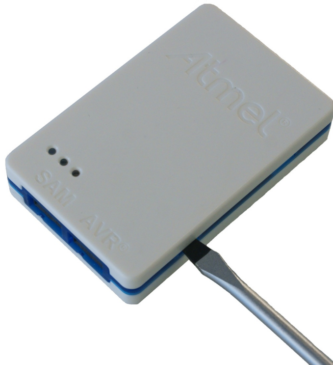
Figure 2-13. Opening the Atmel-ICE (2)
