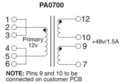
**NOTE:** Pins 9 and 10 to be connected on customer PCB
