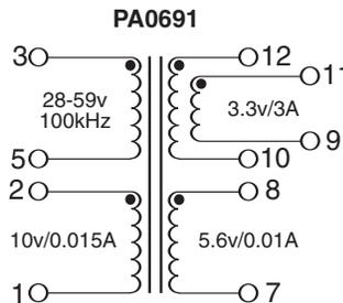
**NOTE:** Pins 8, 9 and 10 to be connected on customer PCB
