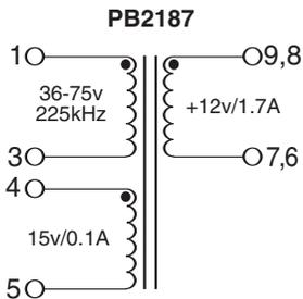
**NOTE:** Pins 9 to 8 and Pins 7 to 6 to be connected on customer PCB
