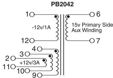
**NOTE:** Pins 2, 3 & 4 and Pins 9, 10 & 11 to be connected on customer PCB
