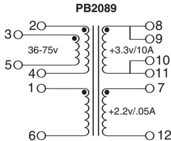
**NOTE:** Pins 2 & 3 and Pins 4 & 5 to be connected on customer PCB
