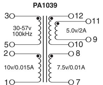
**NOTE:** Pins 8, 9 and 10 to be connected on customer PCB
