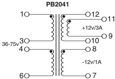
**NOTE:** Pins 12 & 11, Pins 9 & 10, and Pins 3 & 4 to be connected on customer PCB
