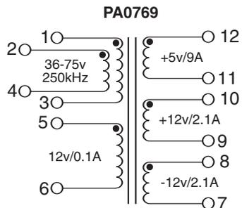
**NOTE:** Pins 1 & 2 and Pins 3 & 4 to be connected on customer PCB
