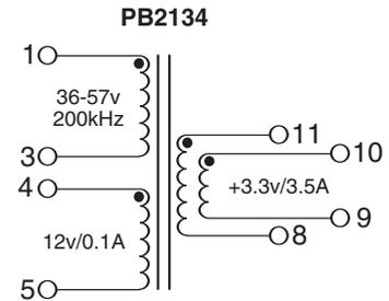
**NOTE:** Pins 10 & 11, Pins 8 & 9 to be connected on customer PCB
