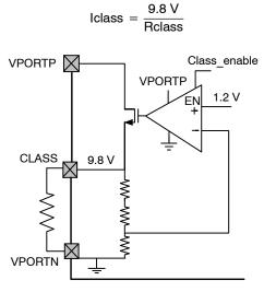
Figure 4. Classification Block Diagram
