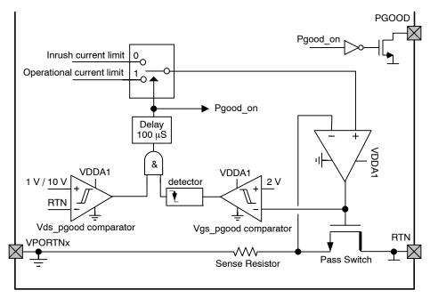
Figure 7. Inrush and Operational Current Limitation Selection Mechanism
