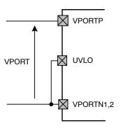
Figure 5. Default Internal UVLO Configuration (NCP1091 only)
