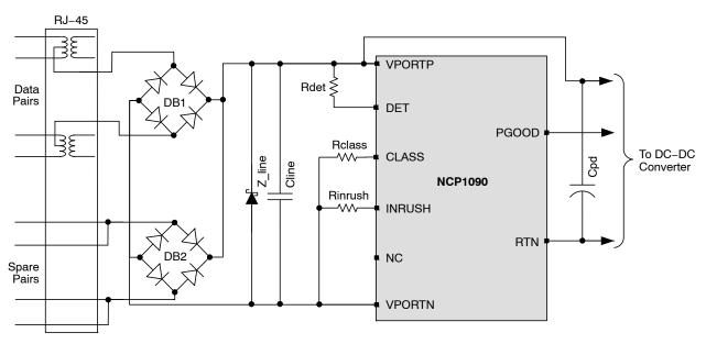
Figure 2. Typical Application Circuit using the NCP1090
