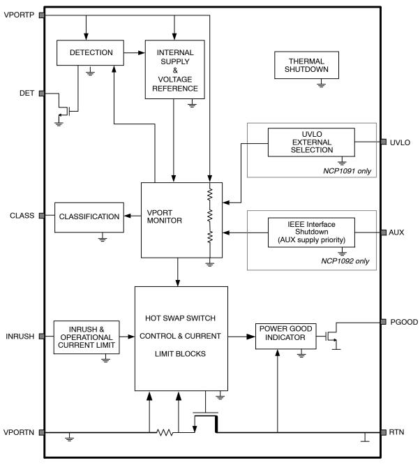
Figure 1. NCP1090/91/92 Functional Block Diagram
