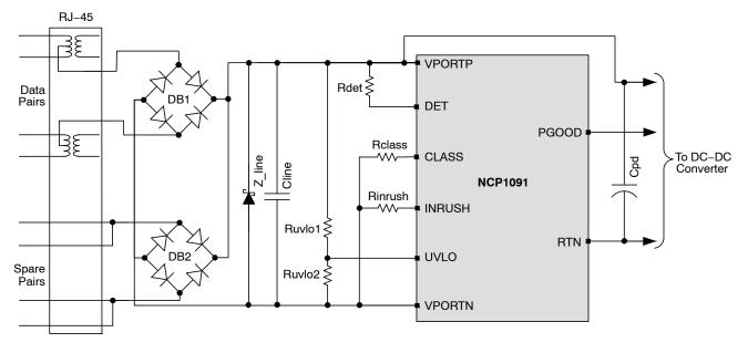
Figure 3. Typical Application Circuit using the NCP1091 with External UVLO Setting
