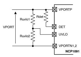
Figure 6. Default Internal UVLO Configuration (NCP1091 only)
