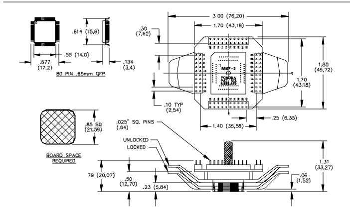
These new test clips provide the user with an easy means to connect instrumentation to the fine pitch QFP chip leads.
