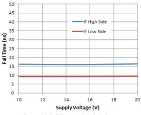
Figure 10. Fall Time vs. Supply Voltage
