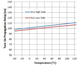
Figure 5. Turn-on Propagation Delay vs. Temperature
