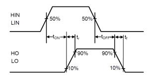
Figure 2. Switching Time Waveform Definitions
