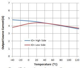
Figure 17. Output Source Current vs. Temperature
