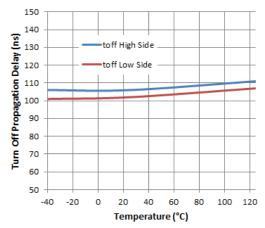
Figure 7. Turn-off Propagation Delay vs. Temperature
