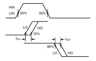
Figure 3. Delay Matching Waveform Definitions
