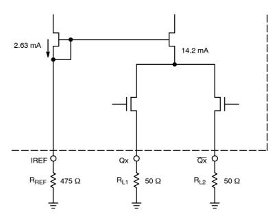
Figure 12. Simplified HCSL Output Structure
