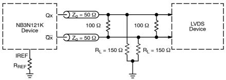
Figure 11. HCSL Interface Termination to LVDS
