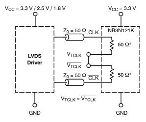
\*RTIN, Internal Input Termination Resistor
