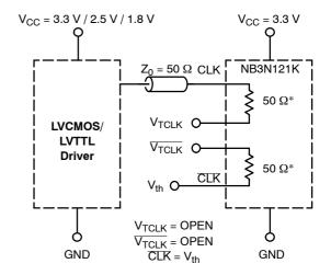
\*RTIN, Internal Input Termination Resistor
