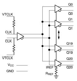
Figure 1. Simplified Logic Diagram
