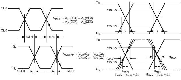
(a) Propagation Delay and Propagation Delay Variation
