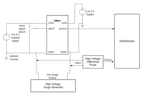
Figure 4.3. Common-Mode Transient Immunity Test Circuit
