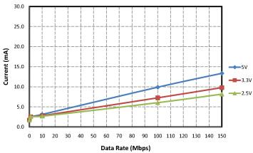
Figure 3.4. Si8631 Typical V<sub>DD1</sub> Supply Current vs. Data Rate 5, 3.3, and 2.5 V Operation
