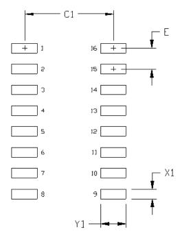
Figure 9.1. PCB Land Pattern: 16-Pin Narrow Body SOIC
