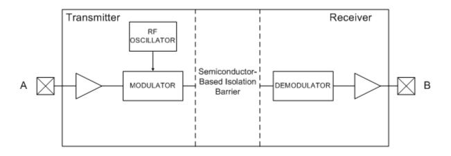
Figure 2.1. Simplified Channel Diagram
