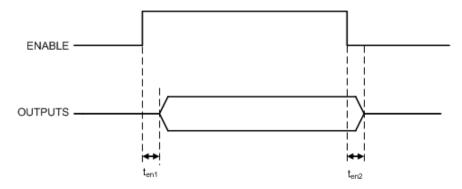
Figure 4.1. ENABLE Timing Diagram
