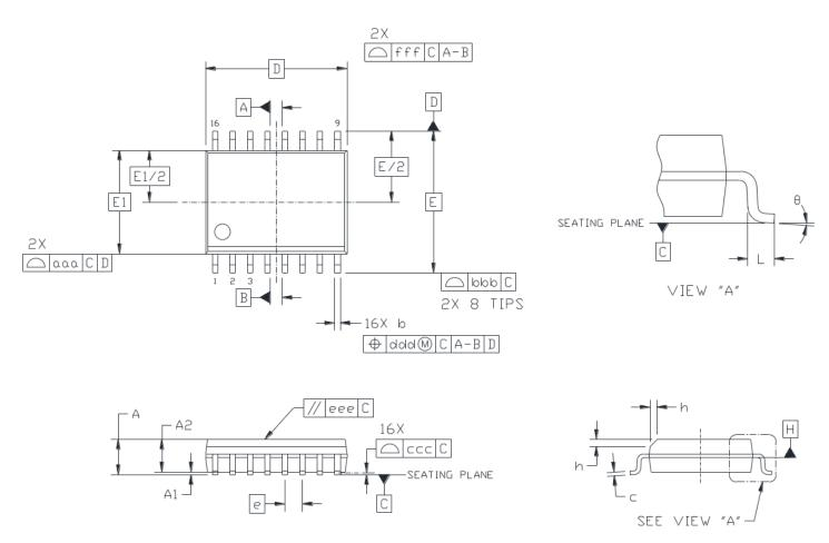
Figure 6.1. 16-Pin Wide Body SOIC
