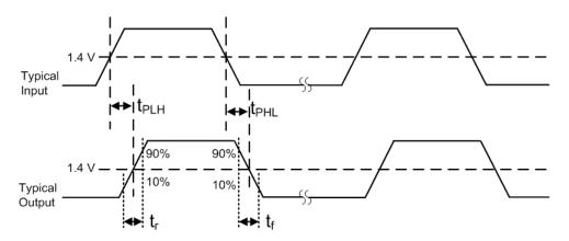
Figure 4.2. Propagation Delay Timing
