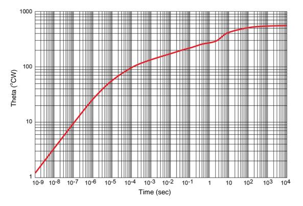
FIGURE 1 Maximum Thermal Impedance (R<sub>0JA</sub>)
