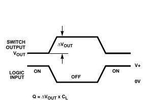
FIGURE 2A. MEASUREMENT POINTS
