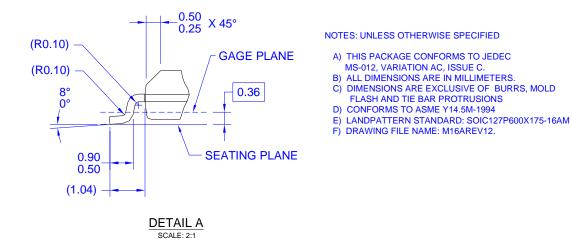
Figure 34. 16-Lead Molded Small Outline Package
