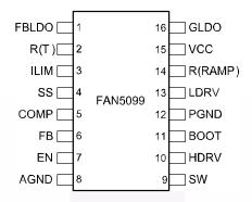
Figure 2. Pin Assignment
