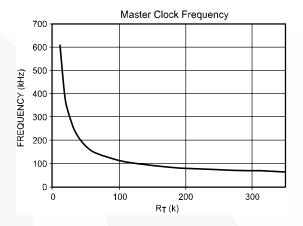
Figure 18. R<sub>T</sub> vs. Frequency
