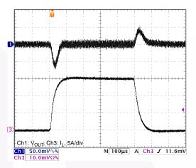
Figure 6. PWM Load Transient (0 to 15A)
