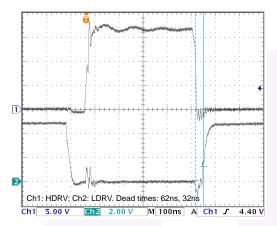
Figure 3. Dead Time Waveform
