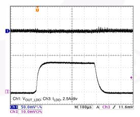
Figure 8. LDO Load Transient (0 to 5A)
