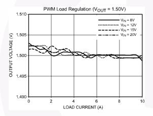
Figure 16. PWM Load Regulation
