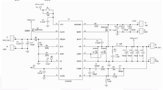
Figure 27. Application Board Schematic
