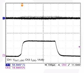
Figure 7. LDO Load Transient (0 to 2A)
