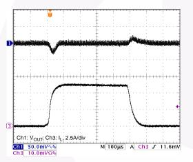
Figure 4. PWM Load Transient (0 to 5A)
