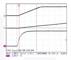
Figure 12. Enable On (I<sub>PWM</sub> = 5A)
