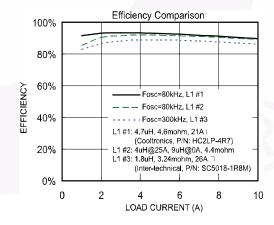
Figure 20. Efficiency Comparison at  $V_{\text{IN}}$ =12V
