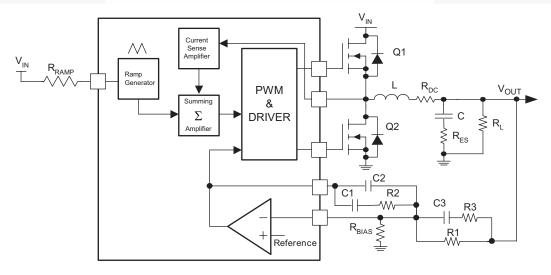
Figure 25. Closed-Loop System with Type-3 Network
