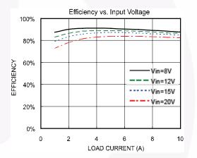
Figure 19. 1.5V PWM Efficiency
