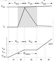
Figure 23. Switching Losses and Q<sub>q</sub>
