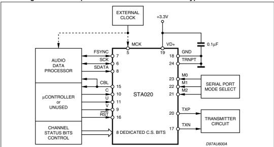
Figure 3. STA020 professional & consumer modes typical connections
