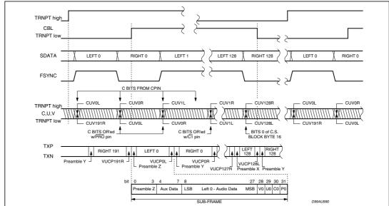
Figure 6. CBL and transmitter timing
