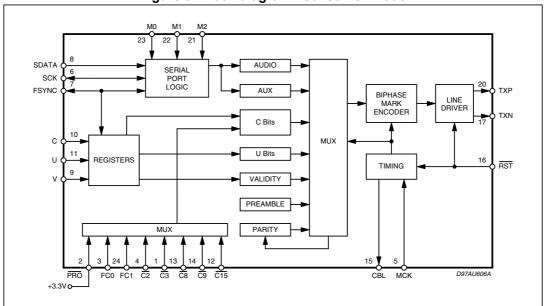
Figure 9. Block diagram - consumer mode
