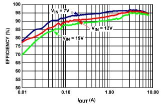
FIGURE 6. CHANNEL 2 EFFICIENCY AT  $V_O = 5V$ , DEM OPERATION. HIGH-SIDE 1xIRF7821,  $r_{DS(ON)} = 9.1m\Omega$ ; LOW-SIDE 1xIRF7832,  $r_{DS(ON)} = 4m\Omega$ ; L = 4.7µH, DCR = 14.3mΩ; CCM  $F_{SW} = 330$ kHz
