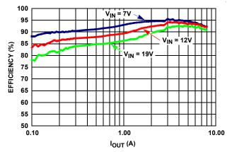
FIGURE 5. CHANNEL 1 EFFICIENCY AT V<sub>O</sub> = 3.3V, DEM OPERATION. HIGH-SIDE 1xIRF7821,  $r_{DS(ON)}$  = 9.1m $\Omega$ ; LOW-SIDE 1xIRF7832,  $r_{DS(ON)}$  = 4m $\Omega$ ; L = 4.7µH, DCR = 14.3m $\Omega$ ; CCM  $F_{SW}$  = 270kHz
