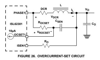
Figure 26 shows the overcurrent-set circuit for SMPS1. The inductor consists of inductance L and the DC resistance (DCR). The inductor DC current  $I_L$  creates a voltage drop across DCR, given by Equation 6:
