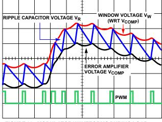
FIGURE 23. MODULATOR WAVEFORMS DURING LOAD TRANSIENT
