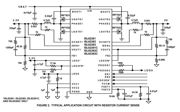
Typical Application Circuits The below typical application circuits generate the 1.05V/15A and 1.5V/15A main supplies in a notebook computer. The input supply (VBAT) range is 5.5V to 25V
