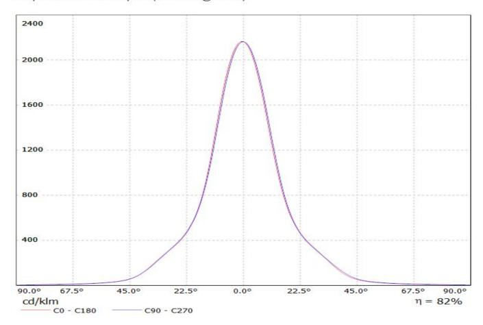
Luminaire: LEDiL Oy CN13113\_LENINA-S-DL\_(SoleriqE30) Eff.82.0% Lamps: 1 x Osram Soleriq E30 (1262.22lm@250mA)
