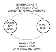
Figure 6. LTC4269-2 Power Good Functional and State Diagram
