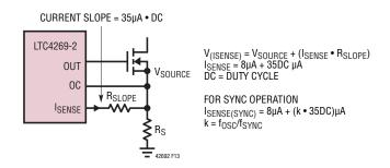
Figure 13. Programming Slope Compensation
