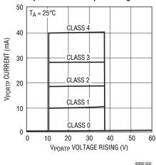
Input Current vs Input Voltage
