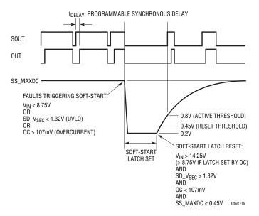
Figure 16. Timing Diagram
