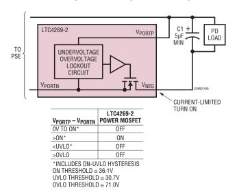
Figure 5. LTC4269-2 Undervoltage and Overvoltage Lockout
