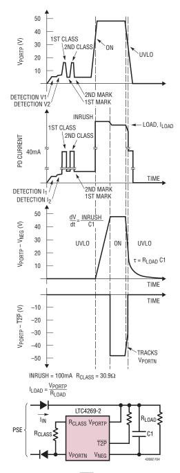
Figure 4.  $V_{NEG}$ ,  $\overline{T2P}$  and PD Current as a Result of 2-Event Classification
