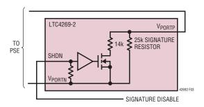
Figure 3. 25k Signature Resistor with Disable
