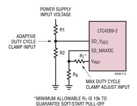
Figure 15. Programming Maximum Duty Cycle Clamp
