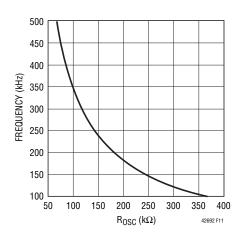
Figure 11. Oscillator Frequency, fosc, vs Rosc
