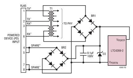
Figure 2. PD Front End Using Diode Bridge on Main and Spare Inputs
