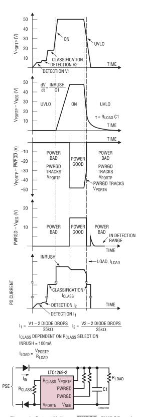
Figure 1. Output Voltage, PWRGD, PWRGD and PD Current as a Function of Input Voltage
