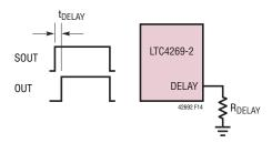
Figure 14. Programming SOUT and OUT Delay: tDFI AY
