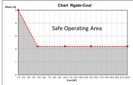
Figure 5. Minimal output series resistance for safe operations
