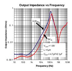
From this graph, you can see the effects of bandwidth and output capacitance. For frequencies <100KHz, the output impedance is dominated by the gain and inductance. For frequencies >100KHz, the output impedance is dominated by the capacitance. A good approximation for transient response can be calculated from determining the frequency of the load step in amps per second:
