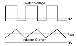
Figure 2. Continuous Operation
