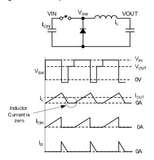
Figure 5. Discontinuous Operation
