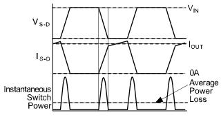
Figure 6. Switching Transition Losses
