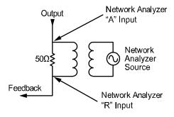
Figure 7. Transformer Injection
