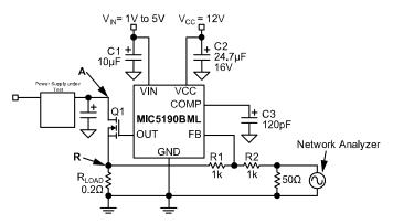
Figure 9. Output Impedance Measurement
