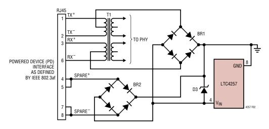
Figure 2. PD Front End Using Diode Bridges on Main and Spare Inputs
