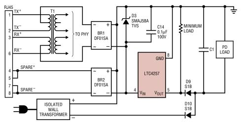
OPTION 3: AUXILIARY POWER APPLIED TO LTC4257 AND PD LOAD
