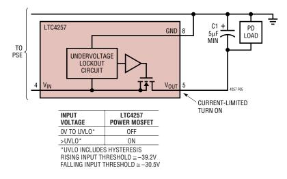
Figure 5. LTC4257 Undervoltage Lockout
