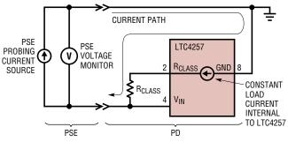
IF PSE PROBING CURRENT < LTC4257 LOAD CURRENT, PD TERMINAL VOLTAGE IS < 15V IF PSE PROBING CURRENT > LTC4257 LOAD CURRENT, PD TERMINAL VOLTAGE IS > 20V 4257 R04
