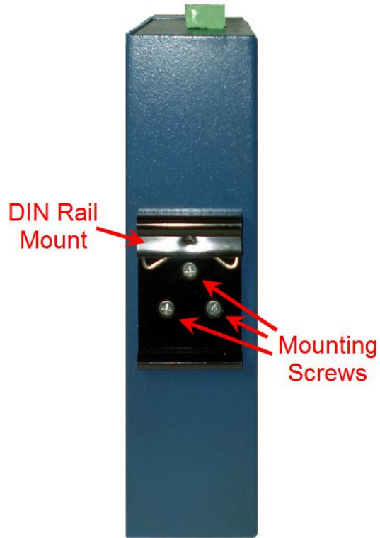
Figure 12. VESR424 with DIN Rail Clip Mounted
