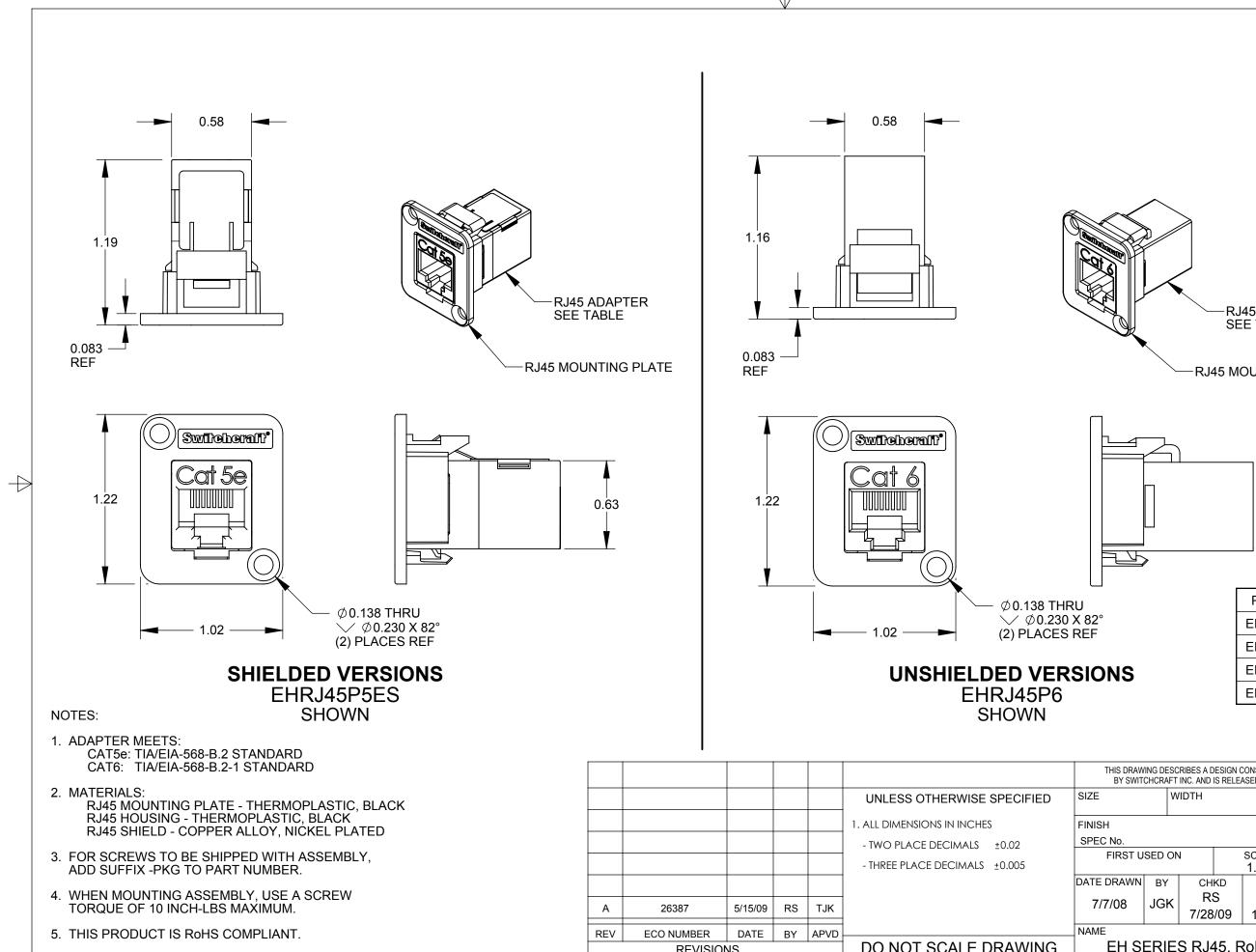
$\emptyset$ 0.945 0.945 Ø0.138 (2) PLACES RECOMMENDED PANEL CUT-OUT -RJ45 ADAPTER SEE TABLE RJ45 MOUNTING PLATE 0.64 PART NUMBER **RJ45 ADAPTER** EHRJ45P5E **CAT5e UNSHIELDED** EHRJ45P5ES CAT5e SHIELDED EHRJ45P6 **CAT6 UNSHIELDED** EHRJ45P6S **CAT6 SHIELDED**
